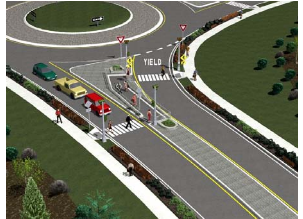
Figure 6. Oblique View of Queue Storage at Unsignalized Staggered/Off-Set Crosswalk
