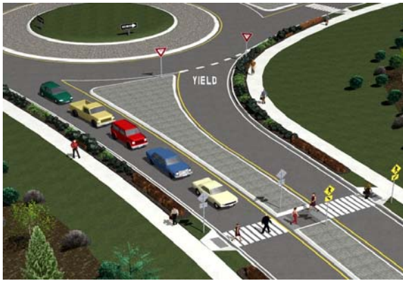
Figure 9. Oblique View of Unsignalized Distal Crosswalk Location Showing Storage of Vehicle Queue Formed When Vehicles Yield to Pedestrians
